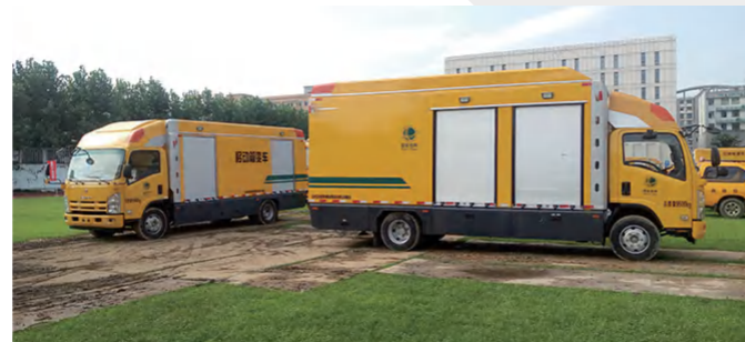
Zhejiang | Off grid distributed energy storage (electric support vehicle) | 304KWh
